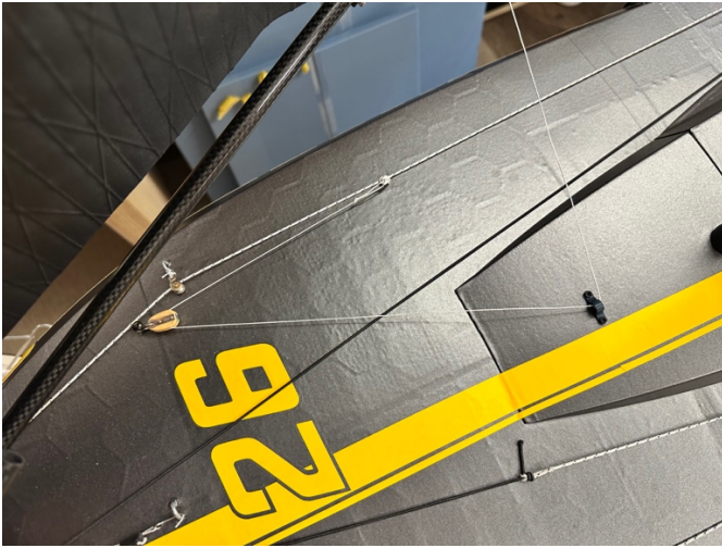
The jib sheet running from the central sheet via a turning block to the jib boom
